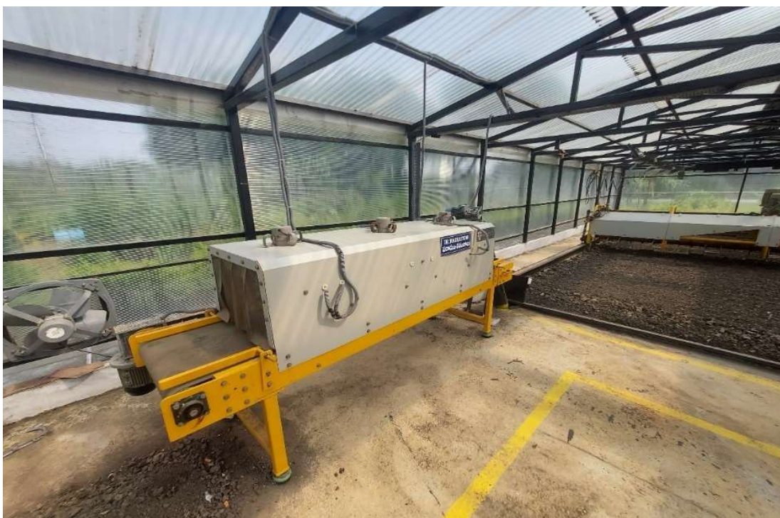
Figure 15: The image here shows drying area within the FSTP, particularly the infra-red drying unit
